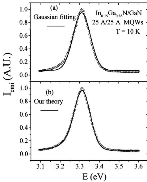
FIG. 3. PL spectrum of the 25 Å/25 Å  $\text{In}_{0.15}\text{Ga}_{0.85}\text{N}/\text{GaN}$  MQWs measured at 10 K together with (a) Gaussian fitting; and (b) fitting by Eq. (5). The fitted parameters  $\sigma_1$  and  $\sigma_2$  are 42 and 88 meV, respectively.
