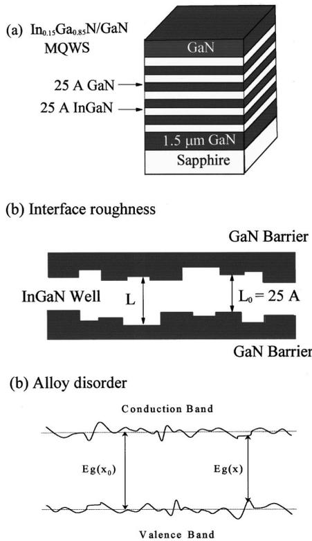
FIG. 1. Schematic diagrams of (a)  $\text{In}_x\text{Ga}_{1-x}\text{N}/\text{GaN}$  MQWs, (b) interface roughness, and (c) energy band-gap fluctuations due to alloy disorder in  $\text{In}_x\text{Ga}_{1-x}\text{N}$  wells.
